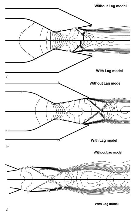
Fig. 4 Mach contours with lag and without lag model: a) NPR = 2.4, b) NPR = 3.8, and c) NPR = 5.4 (maximum value = 1.91, minimum value = 0.15, and interval = 0.3).
