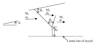
Fig. 5 Shock schematic.
