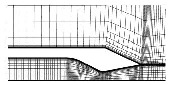
Fig. 1 Grid distribution for the nozzle,  $1216 \times 128$  mesh (for clarity, only every fifth grid line is drawn in each direction).
