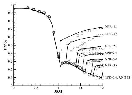
Fig. 2 Comparison of calculated pressure distribution with experimental data<sup>3</sup> (symbols, experiment; solid lines, calculation results with the lag model; dotted lines, calculation results without the lag model).
