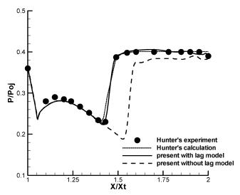
Fig. 3 Comparison of pressure distribution for NPR = 2.4.
