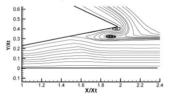
Fig. 6 Streamlines near the rear part of nozzle for NPR = 2.4.
